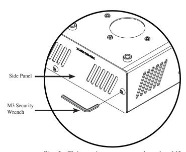
**Step 2.** Tighten these screws using the M5 security wrench.
